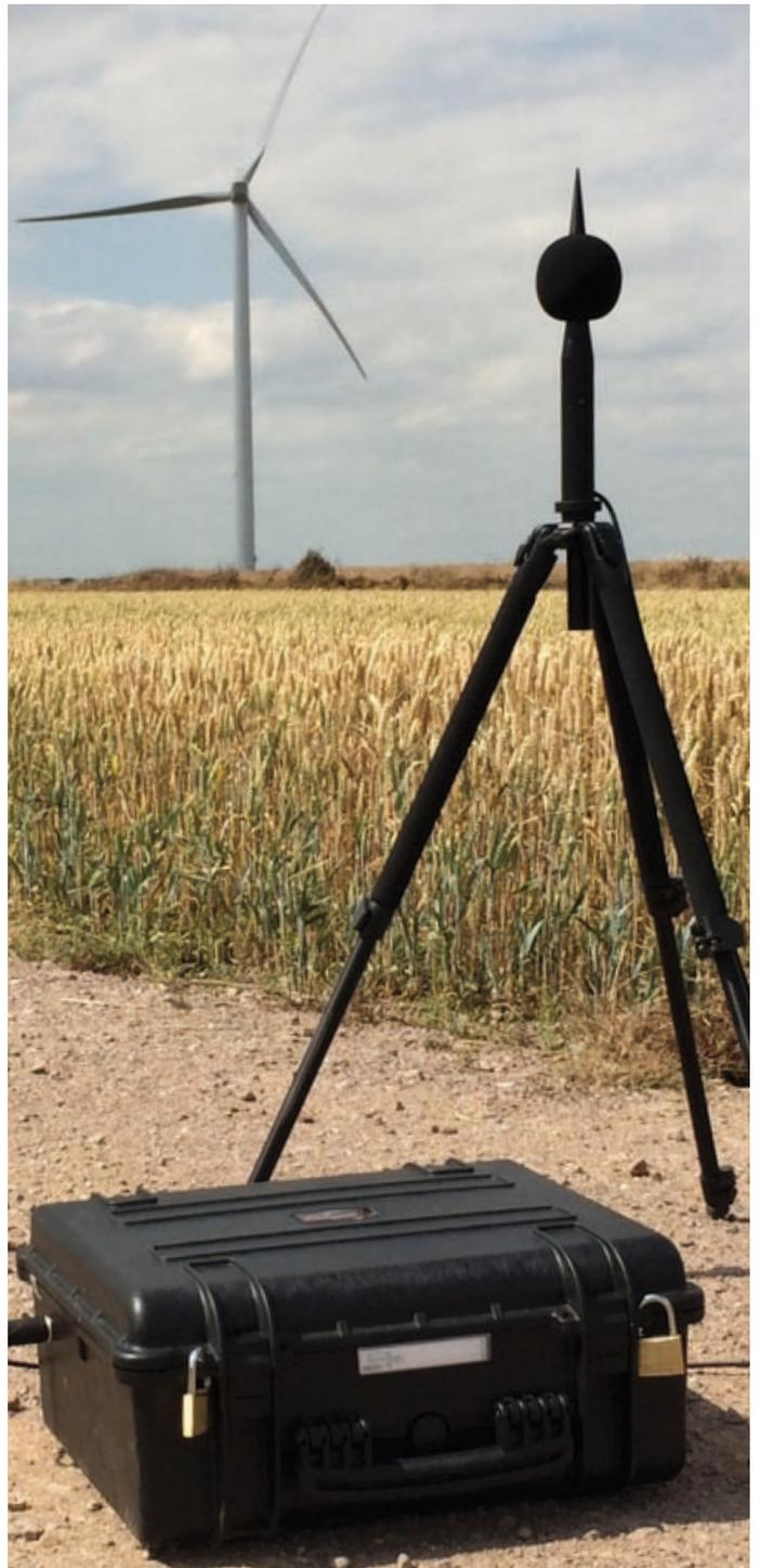
The robust Outdoor Noise Monitoring Solution consists of the XL2 Sound Level Meter, a NetBox with mobile data connection, the heavy duty outdoor case (IP65), extended battery power supply and the outdoor measurement microphone M2230-WP.
